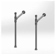
3. Install sink top and bracket according to the sink model. The stone sinks are counterbored on the underside to accept the top 3/8" of the front legs. The collars directly under the sinks do not support any weight. These can be adjusted up against the sink bottom when you are done with the final assembly.
