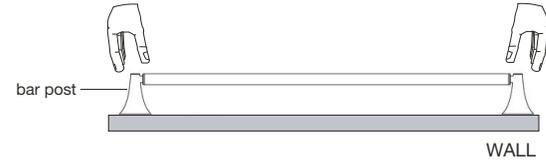
2. Using the Allen key provided, remove the holder post from the mounting post. Press the mounting post against marked post position on the wall and mark the screw hole positions.
