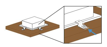
Place sink upside down over the open hole. Slide the brackets over sink edges and fully tighten the screws to lock sink to countertop. **NOTE:** For additional support you may add a bead of caulk to lip of sink before making contact with surface.
