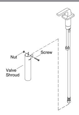
**NOTICE: Risk of product damage.** Hose should not contact or rub on the edges of the valve shroud.
