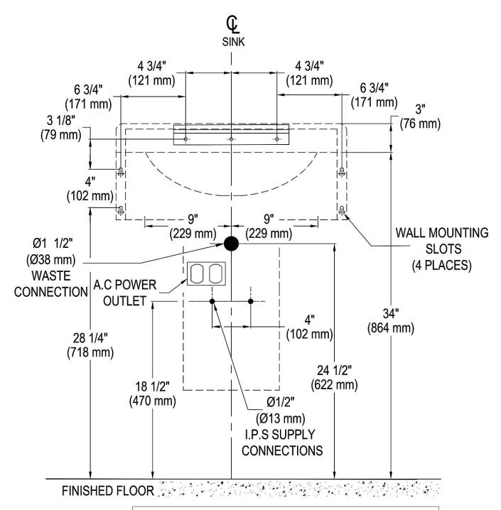
\*NOTE: ALTERING THIS DIMENSION COULD CAUSE SINK TO BECOME NON-ADA COMPLIANT
