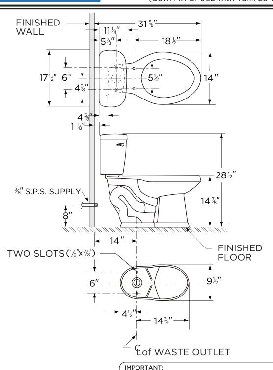
Dimensions of fixtures are nominal and may vary within the range of tolerances established by ASME Standard A 112.19.2.
