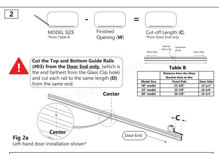
CUTTING FORMULA: FINISHED OPENING - 3-3/8" = FINISHED CUT LENGTH "D" \*for easier installation into the opening, cut off an additional 1/4"
